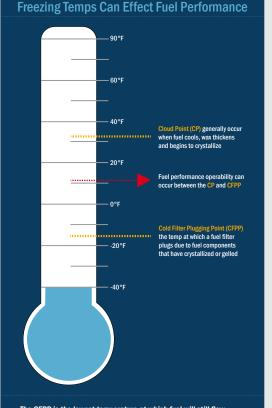
The CFPP is the lowest temperature at which fuel will still flow through a specific filter. The temperatures at which CFPP occurs and the results of fuel additive treatments can vary.
